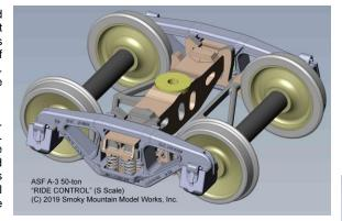
Lubrication is not required to achieve long life or good rolling qualities once installed on a car. If lubrication is desired, use Graphite powder commonly found in the RC plane section of hobby shops ("P84" by Perfect company is what I use). Oil is not recommended because it attracts dirt and can prevent free-rolling axles over time.
